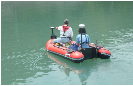
Fig. 2: Terrain measurement using rubber boat, RTK-GPS and sonic depth finder.
