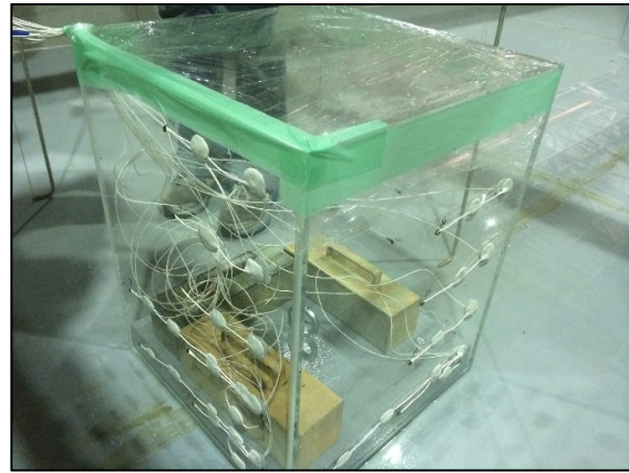
Figure 2. Acrylic box with pressure sensor
