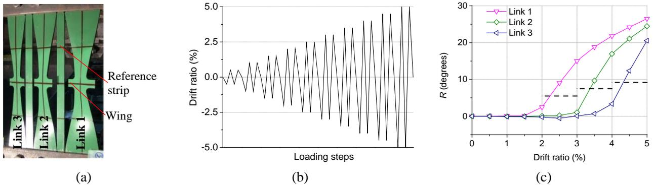
Fig. 2 Torsional deformation under incremental two-cycle loading: (a) test specimen; (b) incremental two-cycle loading; (c) progress of torsional deformation.
