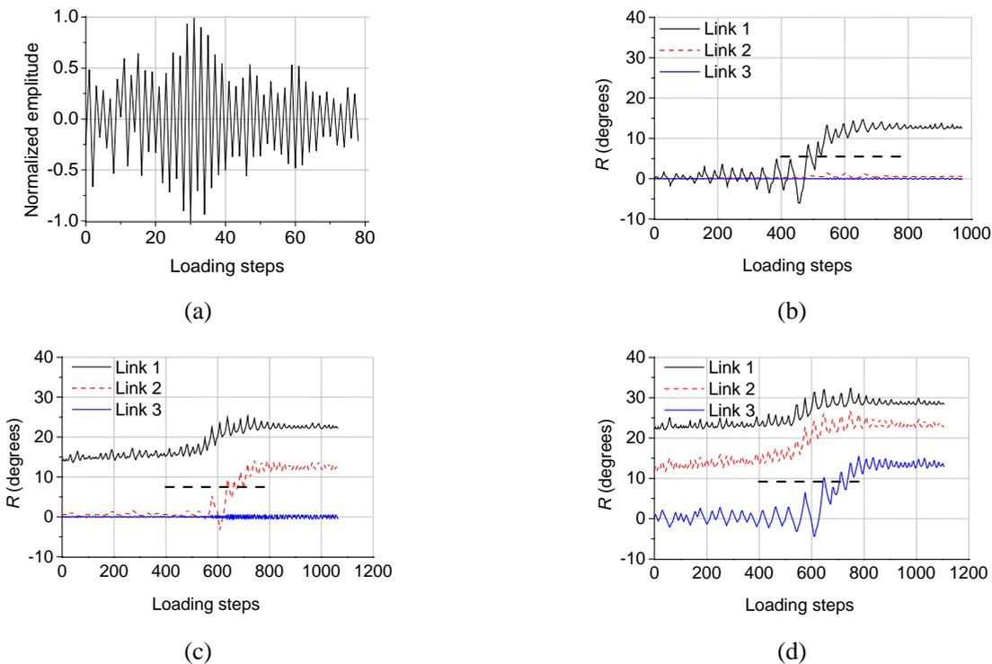
Fig. 3 Torsional deformation under earthquake loading: (a) earthquake loading; (b)-(d) histories of torsional deformation at the largest peak drift ratios of 2.5%, 3.5% and 4.5%, respectively.
