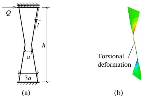
Fig. 1 Double-tapered link: (a) basic dimensions; (b) torsional deformation.
