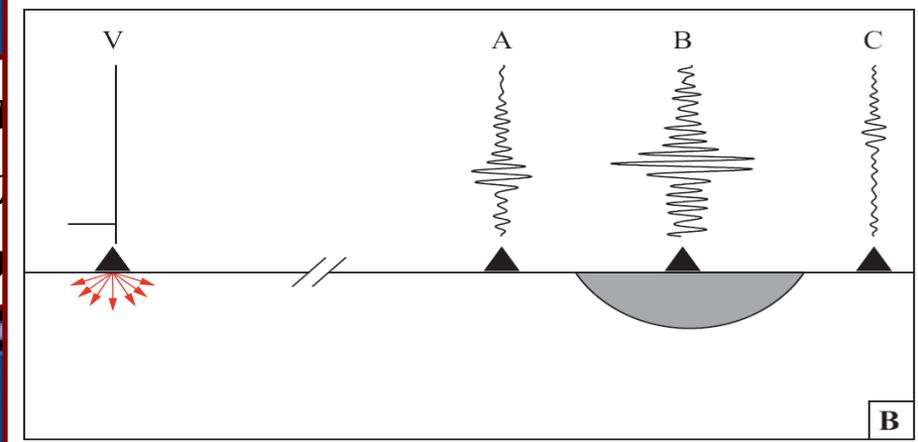
**Active Approach: Deploy instruments and construct virtual earthquake from ambient-field Green's functions.**
