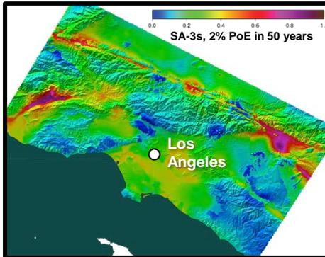
② CyberShake 14.2 seismic hazard model for LA region
