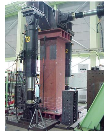
Steel bridge pier test
