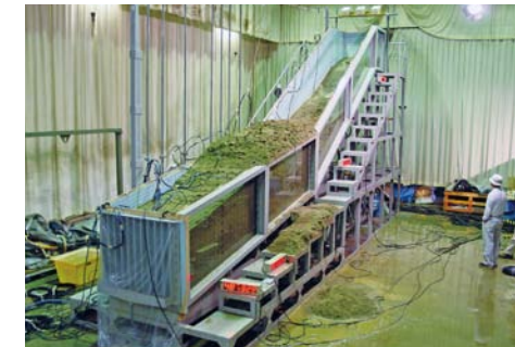
室内降雨崩壊実験 (森林総合研究所の施設を利用) Flume experiment related to rainfall induced shallow landslides (used the equipment in Forestry and Forest Prod. Res. Inst., Tsukuba)
