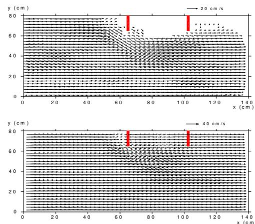
**Fig.1** PIV results for water surface velocity vectors – bandal-like structures (top:non-submerged; bottom:submerged)
