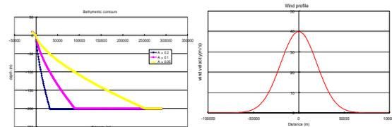
Fig.1 Cross-shore section and wind speed distribution
