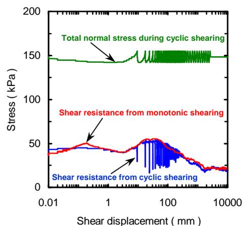
Fig.1. Shear resistance of saturated sand under monotonic and cyclic loading conditions
