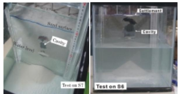
Fig. 2 Wash out through aperture leading to cavity formation in unsaturated sandy backfill
