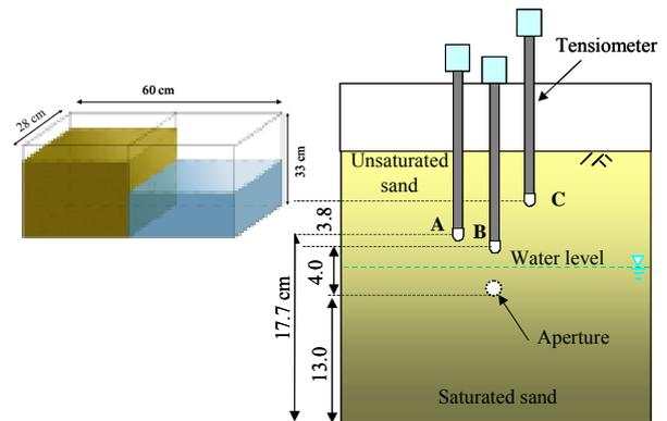
Fig. 1 Apparatus used in experiment
