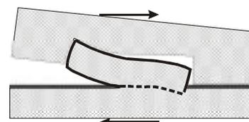
(b) When the maximum shear stress is reached
