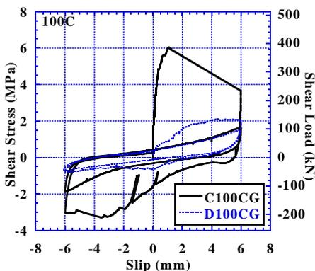
Fig.1 Shear stress-slip relation for a specimen with rectangular shear keys
