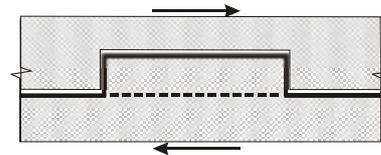
(a) Minor slip due to loss of cohesion
