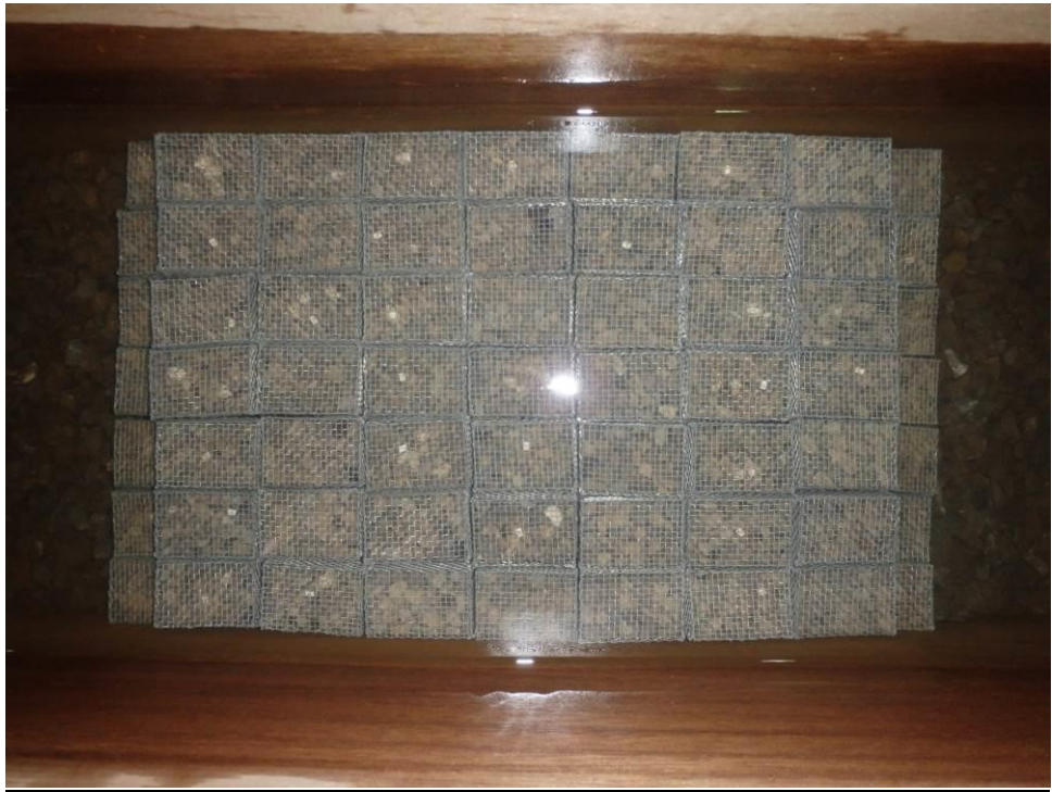
Photo 3A Effect by tsunami action ( no damage, tsunami height=13.7cm, water depth=20cm)
