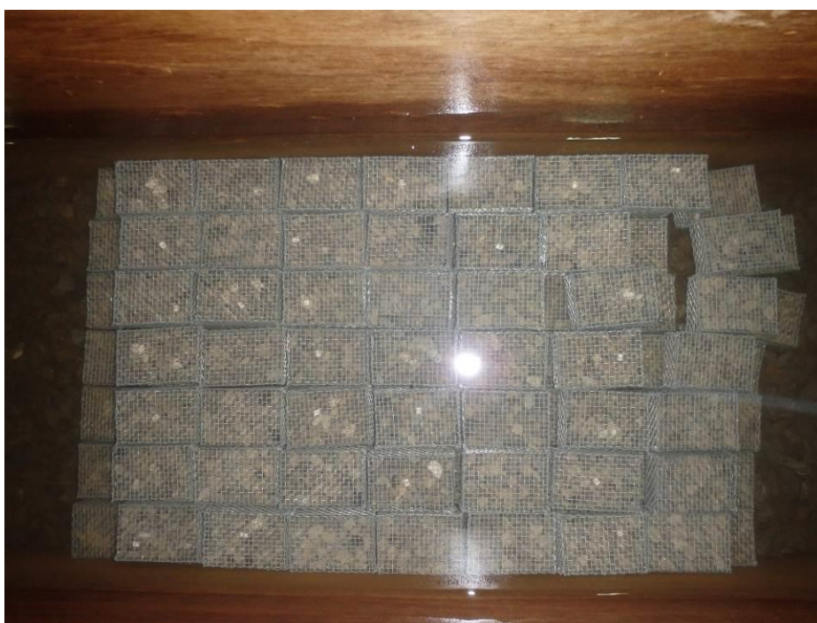
Photo 2A Relocated marine mat due to wave action (waves are acting from left side)
