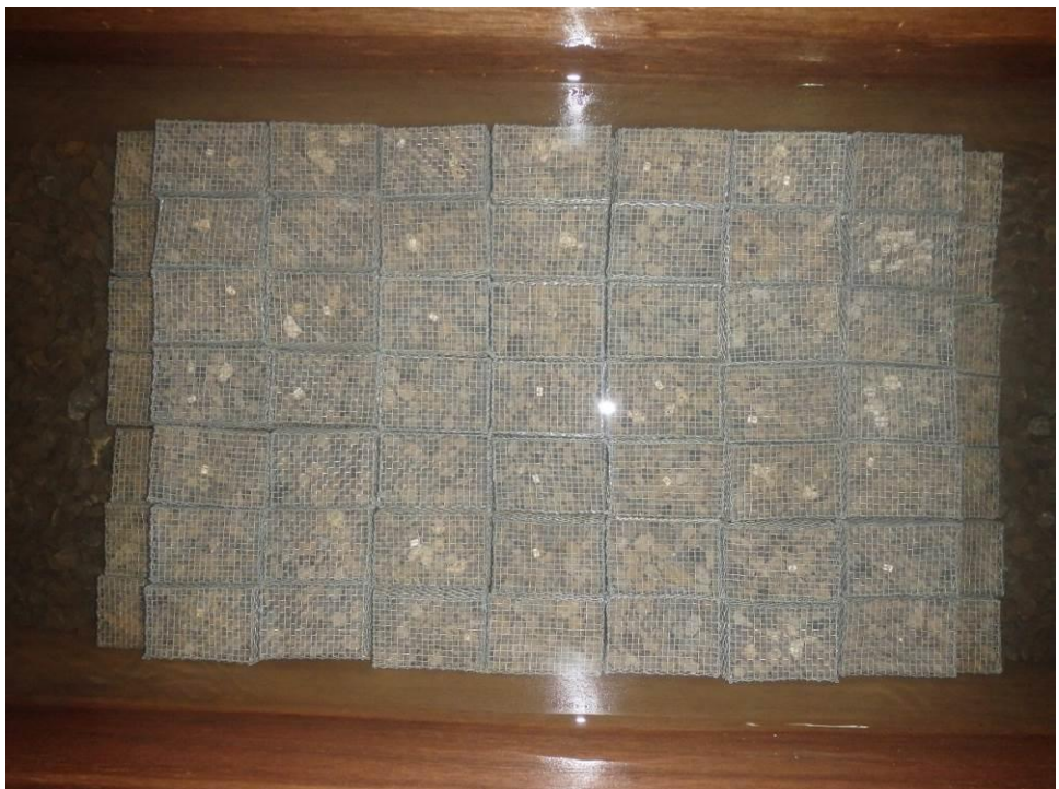
Photo 3A Effect by tsunami action ( no damage, tsunami height=13.7cm, water depth=20cm)
