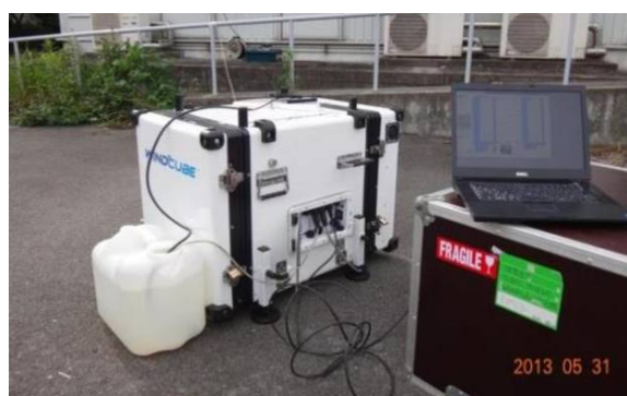
Photo 2 Doppler lidar (WINDCUBE WLS7)
