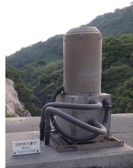
Photo 4 Automatic weight measurement system for volcanic ash
