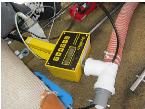
Photo 6 Dust meter: Total, PM10, PM2.5, PM1.0 particles are monitored. Brown tube from the dust meter is connected to the air vent of the plane.
