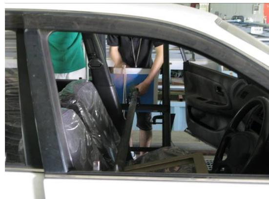
Photo 2 Measurement of force to open the door
