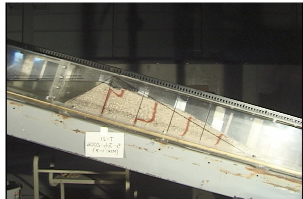
Photo 1 Slope sliding of dam in constant water level in reservoir
