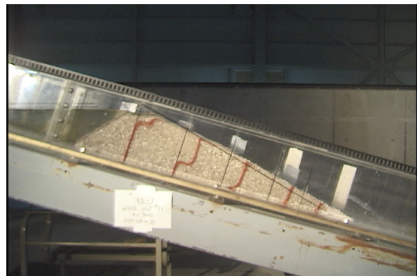
Photo 2 Slope sliding of dam in steady discharge in reservoir
