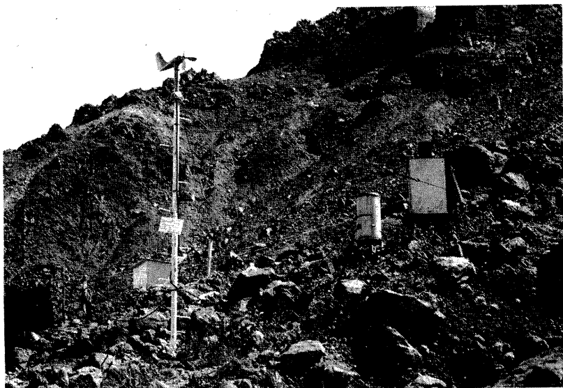
Photo. 1. Propeller anemometer and other equipments in source area (cf. the mark W in Fig. 6 for the location).
