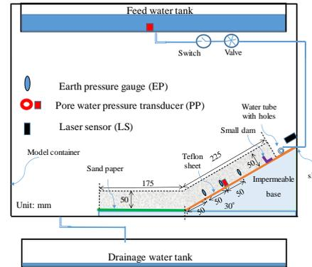
**Fig. 1** Model configuration in prototype scale
