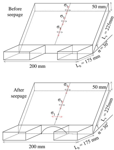
**Fig. 4** Stress transformation in slope model (Test 2)
