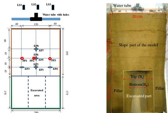
(a) Location of the instrumentations (b) Physical model after preparation
