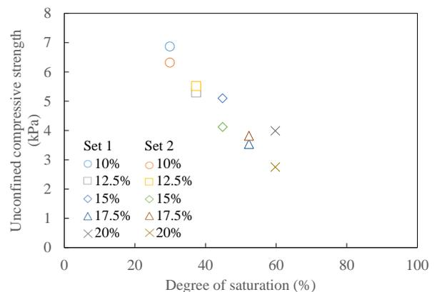
**Fig. 5.** Unconfined compressive strength of Edosaki sand with different degree of saturation
