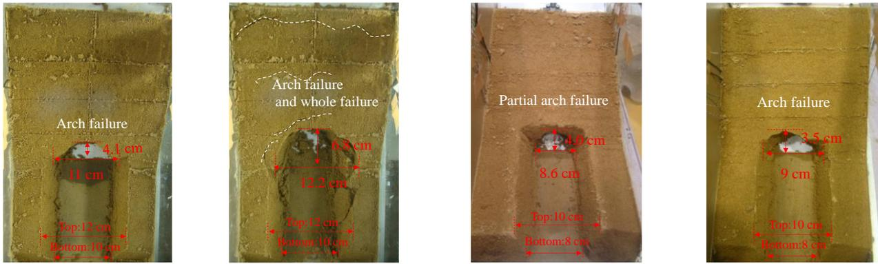
(a) Arch failure due to centrifugal force in Test 1 (b) Whole failure due to seepage in Test 1 (c) Partial arch failure due to seepage in Test 2 (d) Arch failure due to seepage in Test 3
