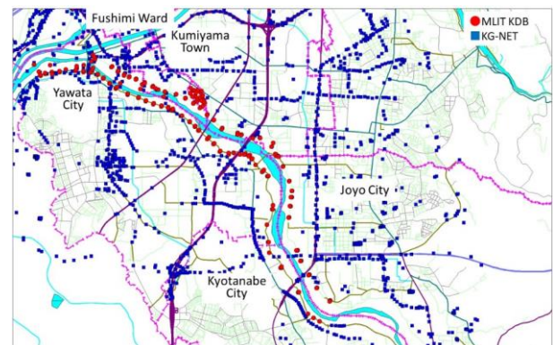
Fig. 1 Distribution of subsoil borehole data of KG-NET and river-bank data of MLIT
