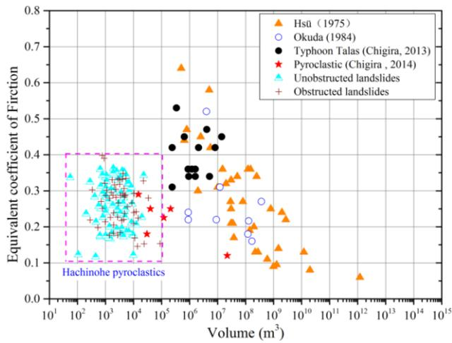
Fig. 4. Equivalent coefficients of friction plotted with landslide volumes. Landslides of pyroclastic deposits are plotted far below the trend of the other landslides.
