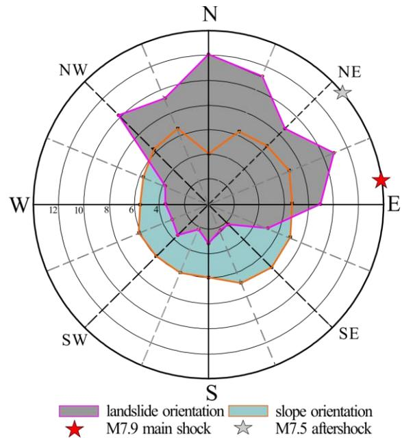
Fig. 5. Normalized distribution of orientation of the slopes (brown line) and landslides (purple line). Stars refer to the relative mean position of the epicenter in M7.9 mainshock (red) and M7.5 aftershock (grey).
