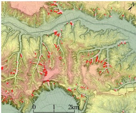
Fig. 1. Distribution of landslides triggered by the M7.9 1968 Tokachi-Oki earthquake.
