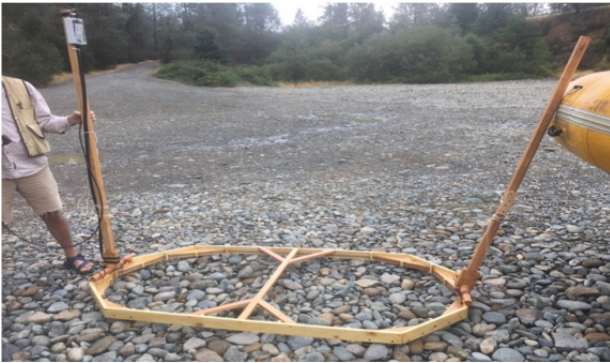
Fig.3: RFID antenna (detector)
