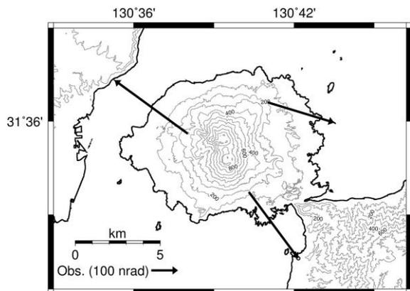
Fig. 3 Observed tilt vectors during the period from 22:07 on November 13, 2017, until 3:00 on the next day. Error ellipses are  $1\sigma$ .
