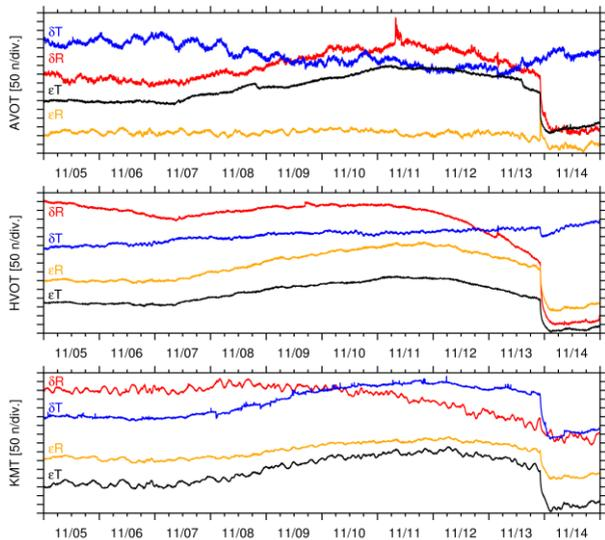
Fig. 2 Tilt ( $\delta$ ) and strain ( $\epsilon$ ) records during the period from November 5 to 14, 2017. R and T are radial and tangential to Minami-dake, respectively.
