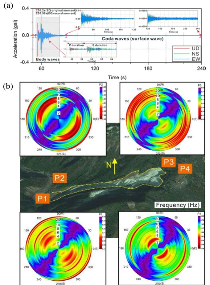
Fig. 2. (a) Time history data for the 3-component acceleration recorded on position P1 from one earthquake event; (b) The amplification effects (average of all the recorded earthquake events in 2015) in frequency domain on different locations. Note: the color scales represent amplified values and the azimuths show the amplified directions.
