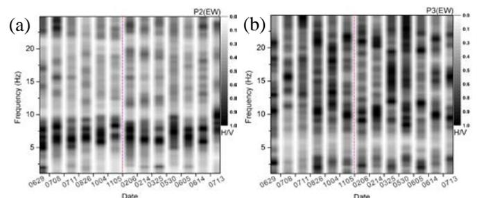
Fig. 3. (a) and (b) the seasonal H/V amplitudes from EW component in frequency bands on landslide deposit area (P2) and slip mass block B (P3), respectively in one year events
