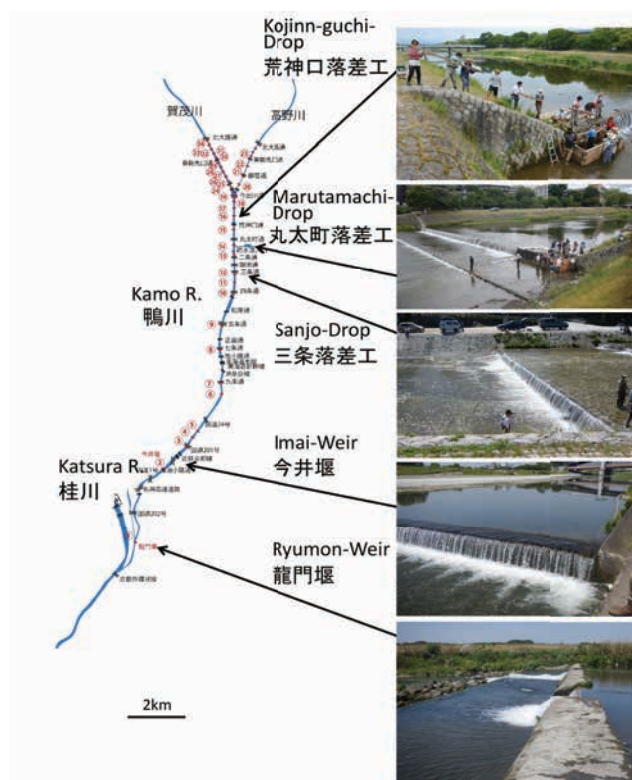
Fig 1 Weirs and drop works hindering up-stream migration of Ayu in the Kamo River.
