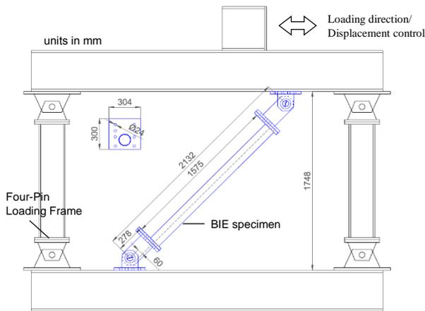
Fig. 3. BIE installed into frame with mechanical pins
