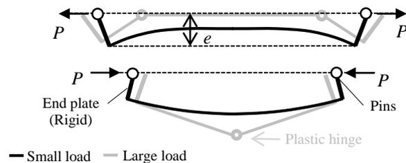
Fig. 2. BIE deformation under tension and compression
