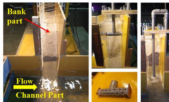
**Fig.2** Side view and details of the eroding jet-pipe.
