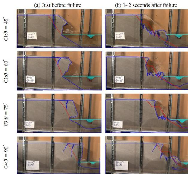
**Fig.3** Results from experimental and model, (a) Just before failure, (b) 1-2 seconds after failure
