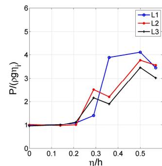
Figure 3. Relationship between solitary wave input and the maximum hydrostatic force
