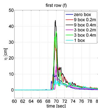
Figure 2. Examples of wave profile at front side of specimen
