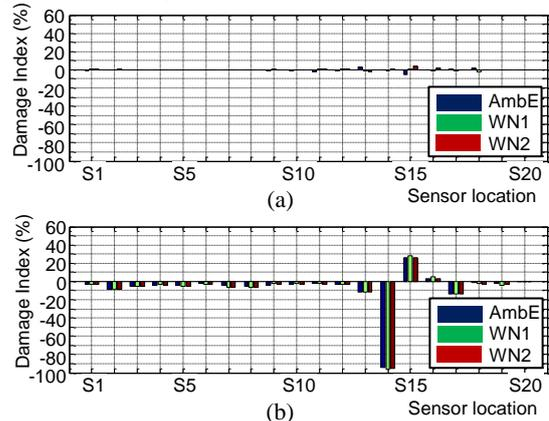
Fig. 3 Damage index: (a) undamaged; (b) damage at B10.
