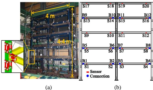
Fig. 1 Steel test frame: (a) overview and removable joints; (b) location of beam connections and sensors.
