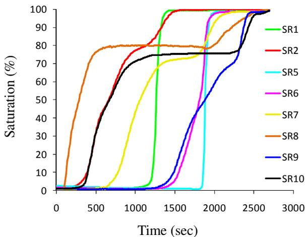
**Fig.1** Experimental moisture profiles at the position of different SRs
