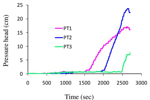
**Fig.2** Experimental air pressure head profiles at the position of different PTs
