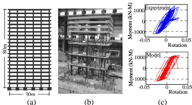
Figure 1 E-Defense test specimen: (a) Prototype building; (b) Test specimen; (c) Hysteretic loop of beam-to-column connection
