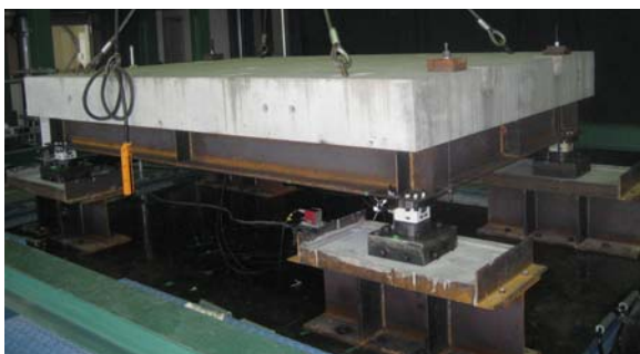
Fig. 1: Rigid frame specimen on the shake table
