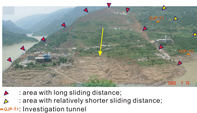
Fig. 1 View of the Qianjiangping landslide from the opposite bank (a: Taken by Y.M. Zhang, July 15, 2003)
