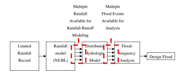
Fig. 1. Concept of the Study Poisson Rectangular Pulse Rainfall Modeling for Design Flood.
