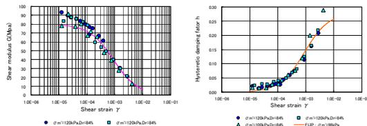
Fig. 3 Sand deformation parameters from test and used in FLIP
