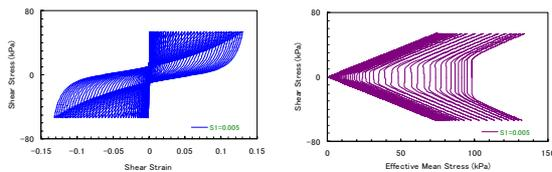
Fig. 4 Cyclic curves of undrained simulation using Flipsim
