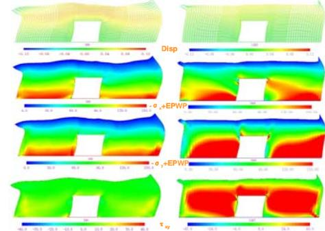
Fig. 8 Normal stress, shear stress with Max x-displacement of RC structure
