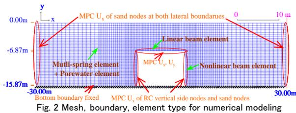
Fig. 2 Mesh, boundary, element type for numerical modeling
